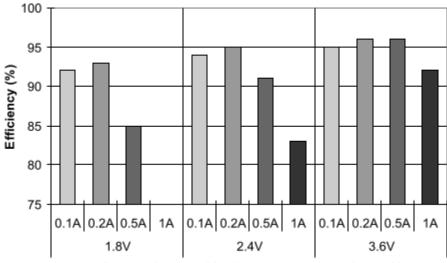
Input voltage and load current, output voltage 5V
